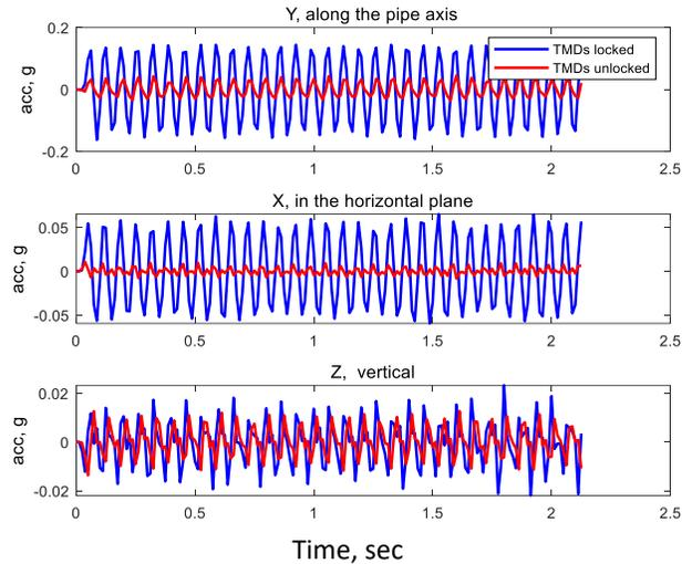
Figure 2 Time traces of acceleration measured close to the X/Y TMD, without (blue) and with (red) the TMDs operational
