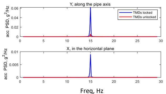
Figure 3 PSDs of acceleration in X and Y directions measured close to the X/Y TMD, without (blue) and with (red) the TMDs operational
