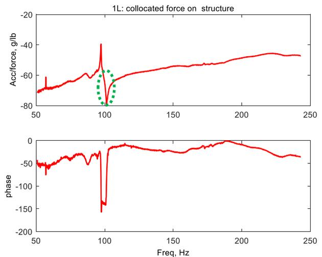
Figure 2 Frequency response function of the structure equipped with the re-tuned DVA
