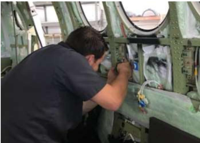
Figure 1 A technician adjusting the active length of the leaf spring of one of the DVAs, by repositioning its mass blocks
