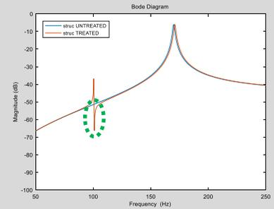
Accurate tuning resulted in absorption of the vibration of the airframe, at the intended offending frequency. The image of Figure 1 shows a technician changing the active length of the leaf springs of a DVA by repositioning its mass blocks.
