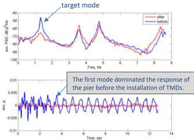
Figure 3 Power spectral densities and time traces of the acceleration measured at the tip of the Pier without (red traces) and with (red traces) the TMDs
