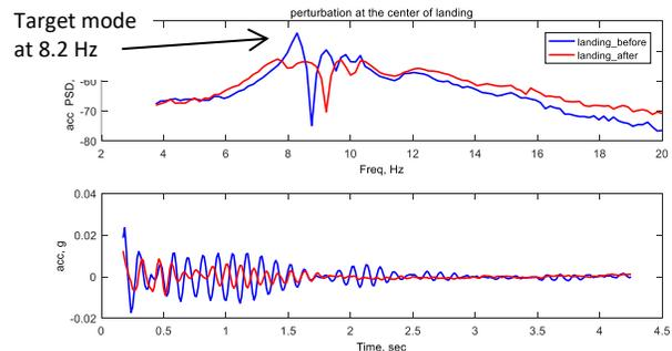
Figure 3 measured vibration without (blue) and with (red) the TMD
