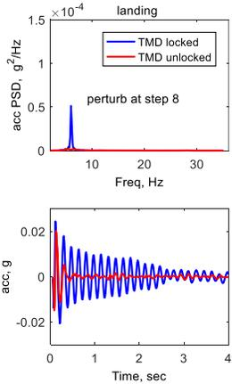
Figure 3 measured vibration with the TMD locked (blue) and unlocked (red)
