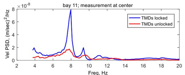
Figure 4 Power spectral density plots of acceleration measured at the center of one of the bays, without (blue) and with (red) the TMDs operational
