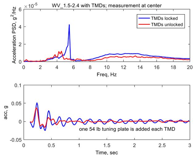
Figure 3 Power spectral density and time traces of acceleration measured, at the center of one of the bays, without and with the TMDs operational
