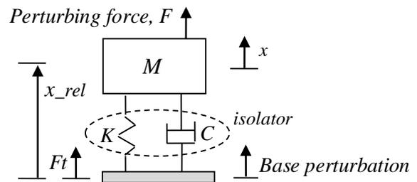
Figure 1 Schematic of an isolated system
