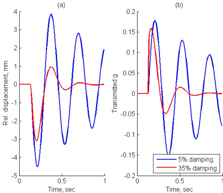
Figure 7 Shock induced relative displacement (a) and transmitted acceleration (b) of an isolated object using soft isolator with sizeable (red traces) and negligible (blue traces) damping
