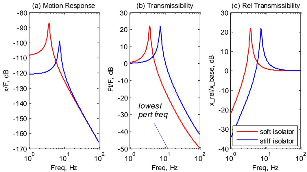
Figure 3 Motion response (a), transmissibility (b) and relative transmissibility (c) frequency response functions for an isolation system with low stiffness (red) and high stiffness (blue)
