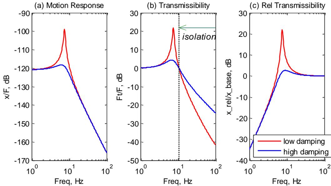
Figure 2 Motion response (a) transmissibility (b) and relative transmissibility (c) frequency response functions for an isolation system with low damping (red) and high damping (blue)
