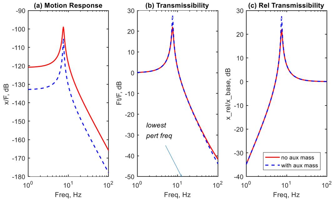
Figure 5 Motion response (a), transmissibility (b) and relative transmissibility (c) frequency response functions for an isolation system without (red/solid line) and with (blue/dashed line) added mass
