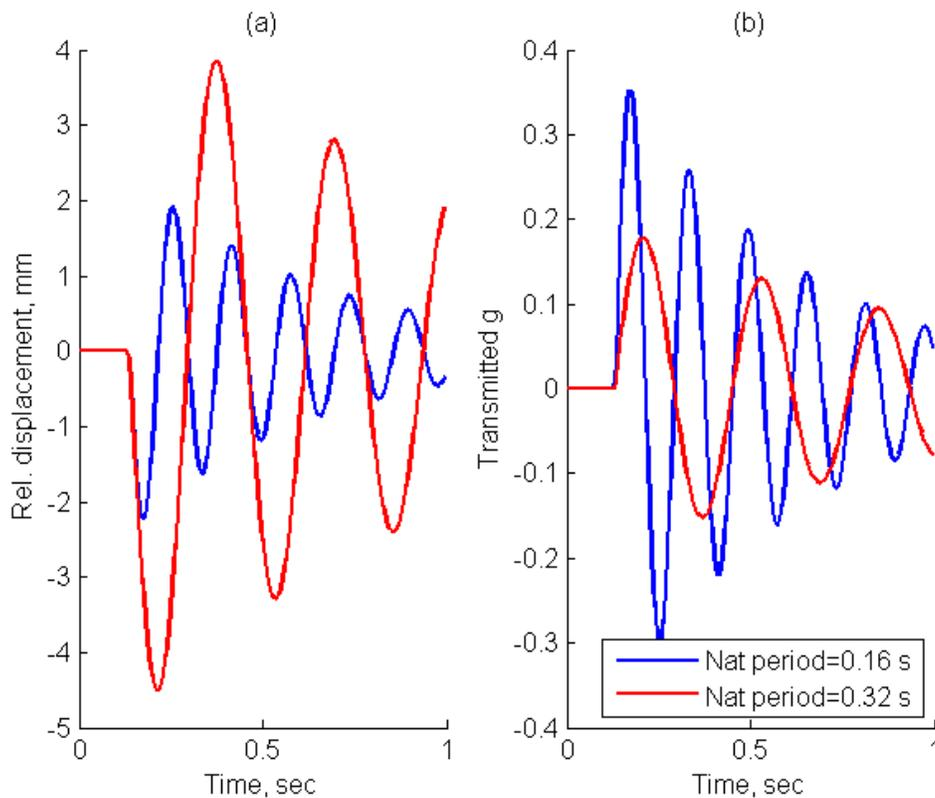
Figure 6 Shock induced relative displacement (a) and transmitted acceleration (b) of an isolated object using soft (red traces) and stiff (blue traces) isolators with negligible damping
