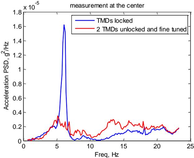
Figure 3 Power spectral density traces of the floor acceleration measured without and with the TMDs operational
