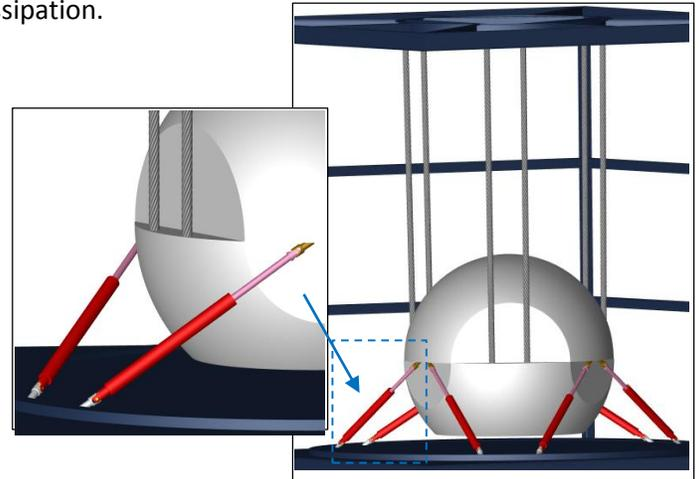
Figure 1 A pendulum tuned mass damper (PTMD)
