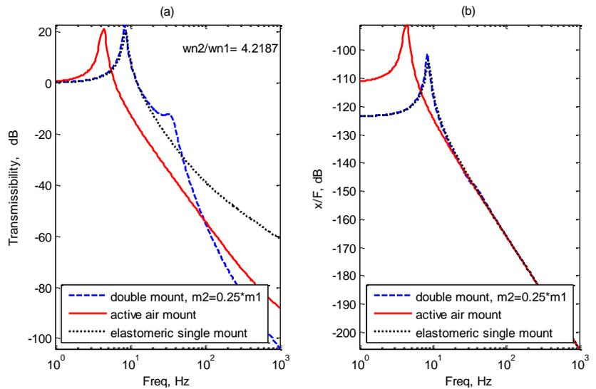
Figure 2 Comparison of transmissibilities (a) and motion of the machine (b) using single mounting (black/dotted line), double mounting (blue/dashed line) and active air mounting
