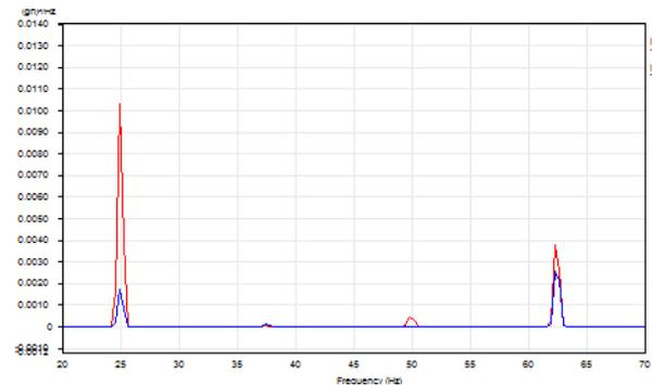
Figure 2 Acceleration power spectra of measured at one of the mounting feet, before (red) and after (blue) the tuned absorbers installation.
