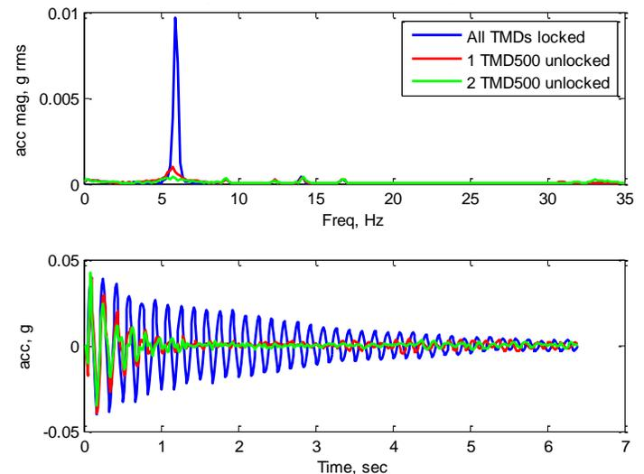
Figure 3 Linear spectra and time traces of acceleration measured without and with the TMDs operational
