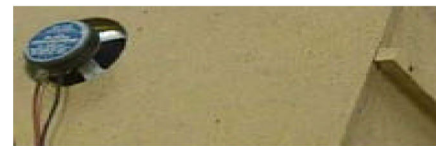
Figure 2. Active Helmholtz resonator installed on an enclosure
