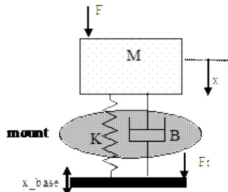
Figure 1 A simple mounting system
