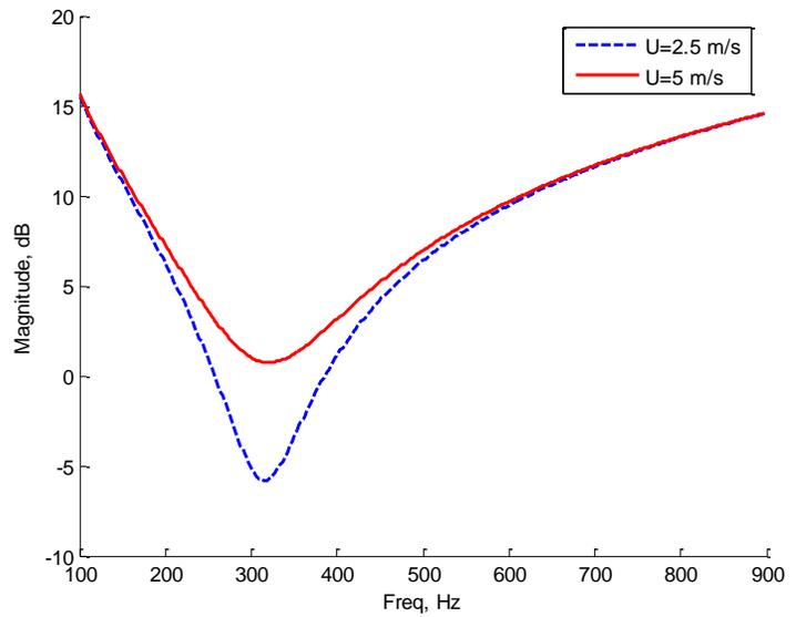
Figure 2 The impedance of a 1/8" hole diameter, 1.5% porosity perforation, and 2" backing at two bias flow velocities
