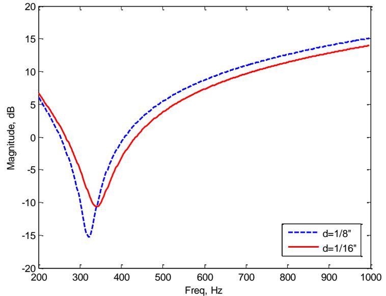
Figure 1 the impedance of two different diameter perforations with 1.5% porosity and a backing space of 2 inches
