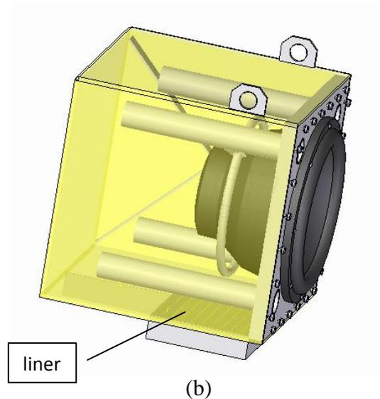
Figure 3 First axial standing wave of the cabinet (a) and an acoustic liner (b) for dampening it
