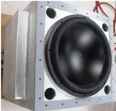
Figure 1 High temperature, low-frequency loudspeaker
