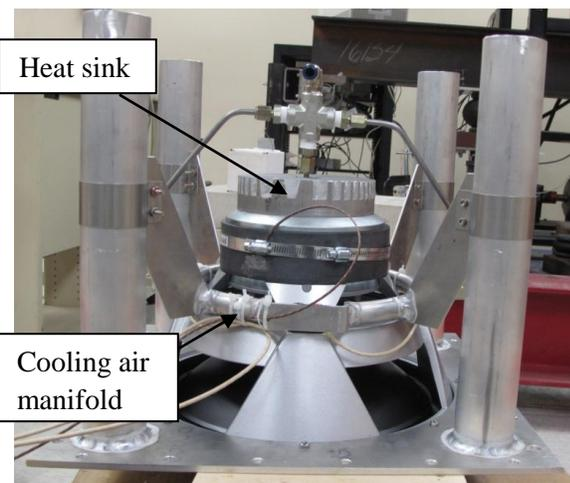
Figure 4 Port and driver assembly
