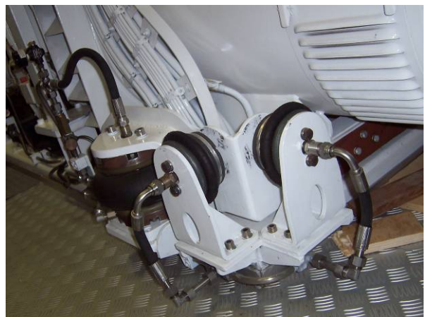
Figure 2. One mounting foot of a diesel generator isolated by DEICON's Computer Controlled Air Isolation System
